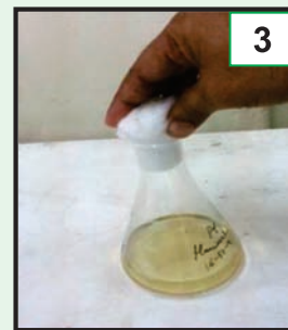
3 Close flask mouth with cotton plug
